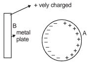
The given diagram shows induction on sphere Q.126 (3) (metallic) due to metal plate.
