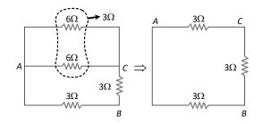
So the equivalent resistance between points A and B
