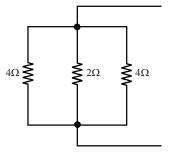
$$\Rightarrow \frac{1}{R_{eq}} = \frac{1}{4} + \frac{1}{2} + \frac{1}{4} \Rightarrow R_{eq} = 1\Omega$$
