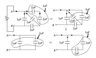
Hence equivalent capacitance between A and B is 2µF.
