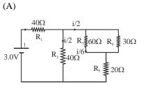
Power dissipate in  $R_1$  is maximum as its current is maximum and its resistance is also 40 $\Omega$  which is higher than  $R_5R_4$ .
