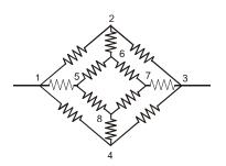
due to input output symmetry, here no current passes through resistance 2 to 6 and 4 to 8. Equivalent circuit is
