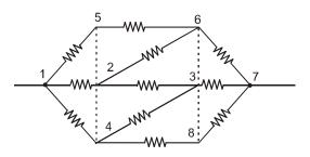
due to input output symmetry potential at point 2, 4, 5, are equal and potential at point 3, 6, 8 are equal
