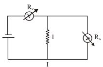
Rv = Resistance of voltmeter RA = Resistance of ammeter
