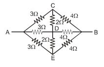
Due to input symmetry potential drop in AC, AD and AE part is same. Therefore potential at C,D and E point is same.
